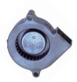
**DC blowers** are used in equipments of air-conditioning and media technology primarily. The housing and the impeller consist of reinforced plastic material. The brushless DC motor is provided with precision ball bearings from NMB's own production. Furthermore the blowers are equipped with inverse-polarity and blocking protection with automatic restart. Tacho signal, locked rotor signal are available on request.
