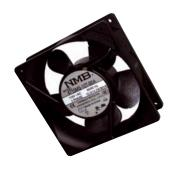
**AC axial fans** with aluminum housing. The impeller consists of reinforced plastic material or metal. A shaded pole motor or condenser motor is provided with precision ball bearings from NMB's own production. The standard direction of flow is blowing, sucking as an option.
